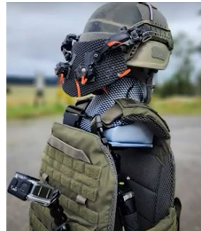
Figure 2. Army helmet with Pelta-6 attachment on test mannequin equipped with Blast Gauge Sensors. JBLM May 2024
