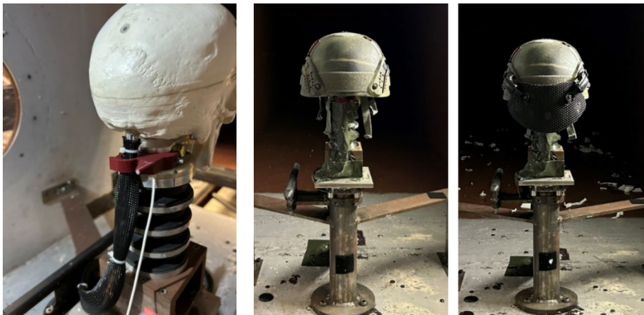
Figure 10. Skull Headform blast wave tests conducted, with and without Pelta-6.
